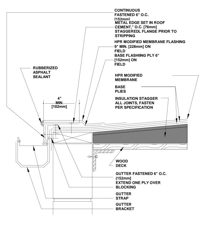
ALL PLIES SET IN MODIFIED COLD ADHESIVE SEE SPECIFICATIONS FOR SURFACING
