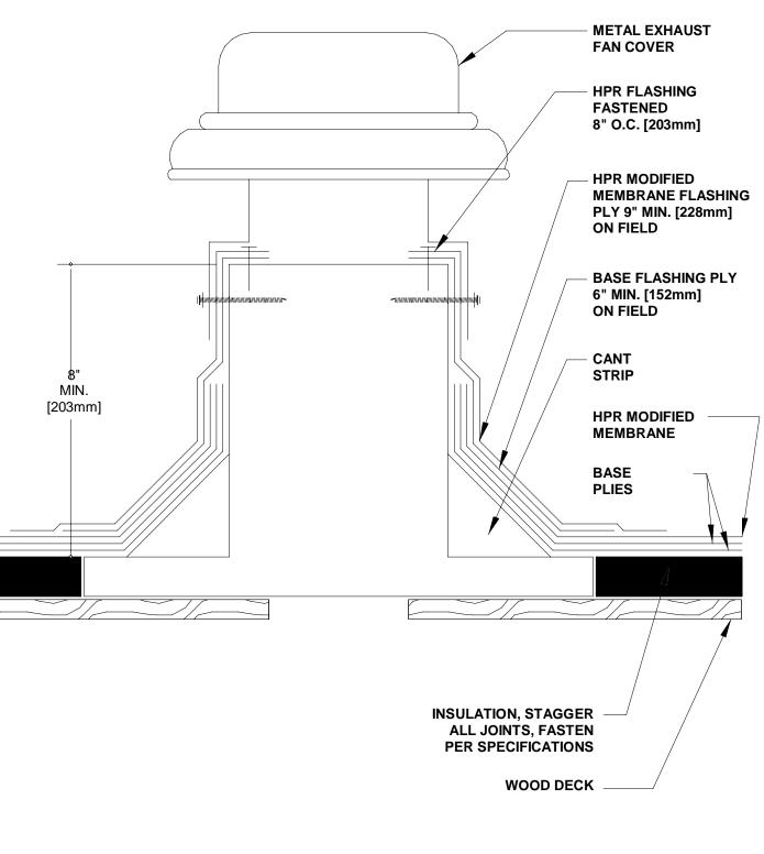
ALL PLIES SET IN MODIFIED COLD ADHESIVE SEE SPECIFICATIONS FOR SURFACING
