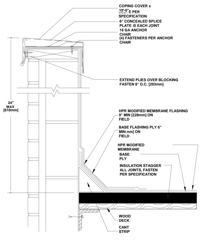
ALL PLIES SET IN BITUMEN SEE SPECIFICATIONS FOR SURFACING
